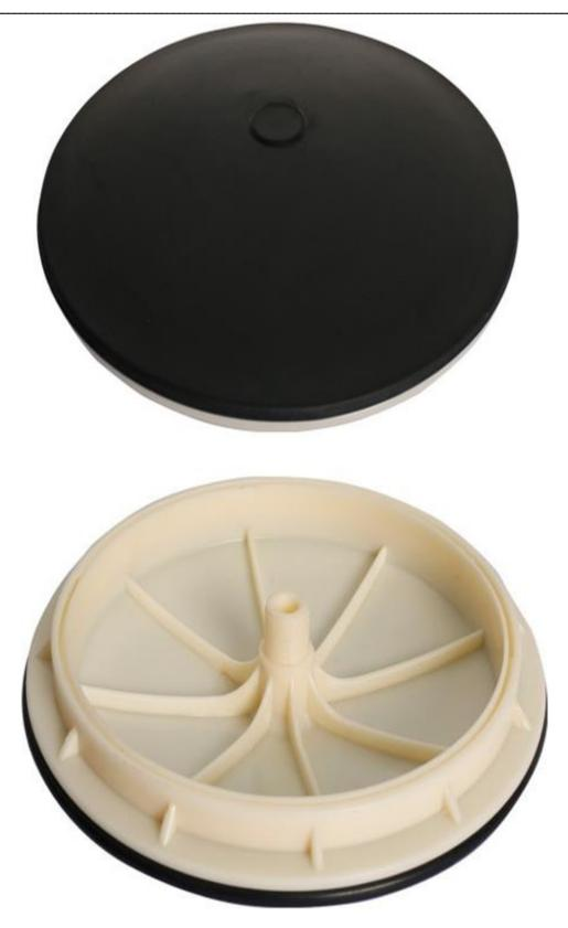
The Fine Bubble Disc Diffuser are designed with an arch surface so that there is minimum accumulation of MLSS and debris on the surface.
